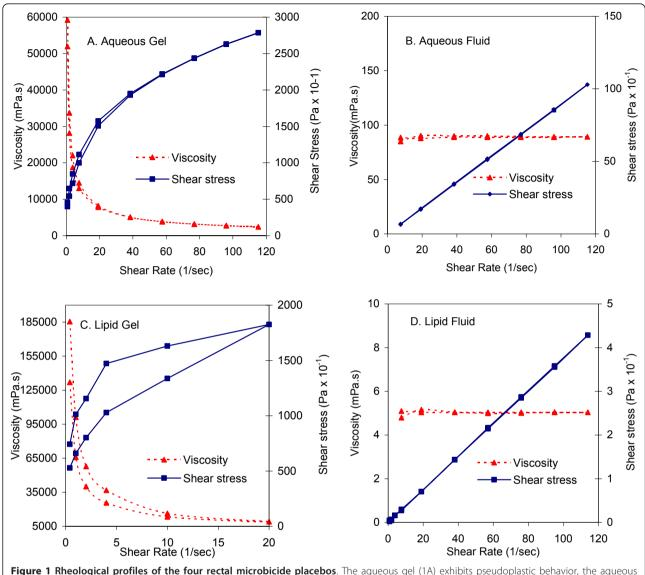
**Figure 1 Rheological profiles of the four rectal microbicide placebos**. The aqueous gel (1A) exhibits pseudoplastic behavior, the aqueous fluid (1B) exhibits Newtonian behavior, the lipid gel (1C) is thixotropic, and the lipid fluid (1D) is Newtonian.
